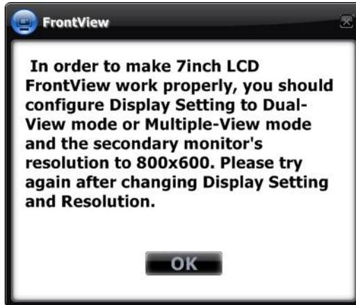
6. Make sure that iMON OEM Touch LCD is matched to secondary monitor with 800\*600 resolution in Dual-View mode. If Touch LCD's resolution is not 800\*600, warning window pops up and advises you to change resolution to 800\*600 (60Hz).
