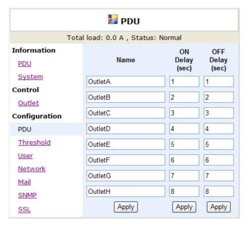
**Note**: After PDU is plugged into main power, PDU system will start to sequentially turn on the output socket according to the pre-set delay time in PDU web interface. The factory default setting for delay time is one second for each outlet; therefore the 8 ports PDU will take 8 seconds, 24 ports PDU will take 24 seconds to complete start-up procedure.
