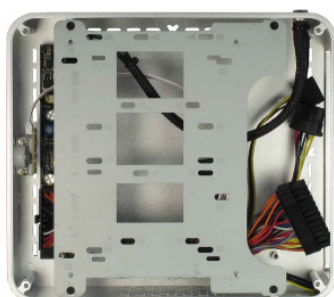
ITX Q-6 with opened side panel (incl. HDD-Tray)
